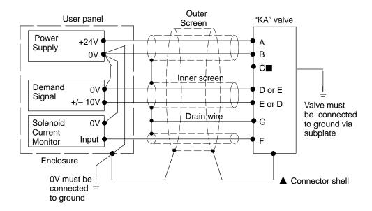
■ Solenoid current monitor voltage (pin F) will be referenced to the KA valve local ground. A "local ground" (pin C) is provided for optional use by differential input customer supplied electronics.
