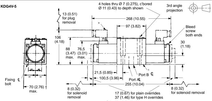
u Electrical plug connections (without indicator light) to ISO 4400/DIN 43650. Must be separately ordered by part number(s).
